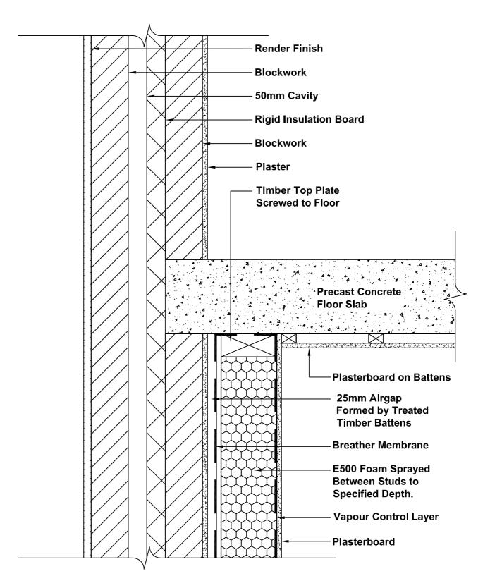
INTERNAL DRYLINING (VERTICAL SECTION -INTERMEDIATE FLOOR BETWEEN APARTMENTS)
