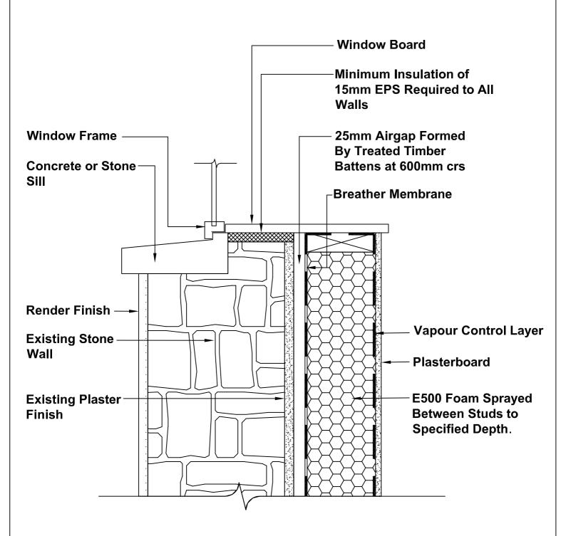
INTERNAL DRYLINING OF EXISTING MASONRY WALLS SILL DETAIL (PLAN SECTION)
