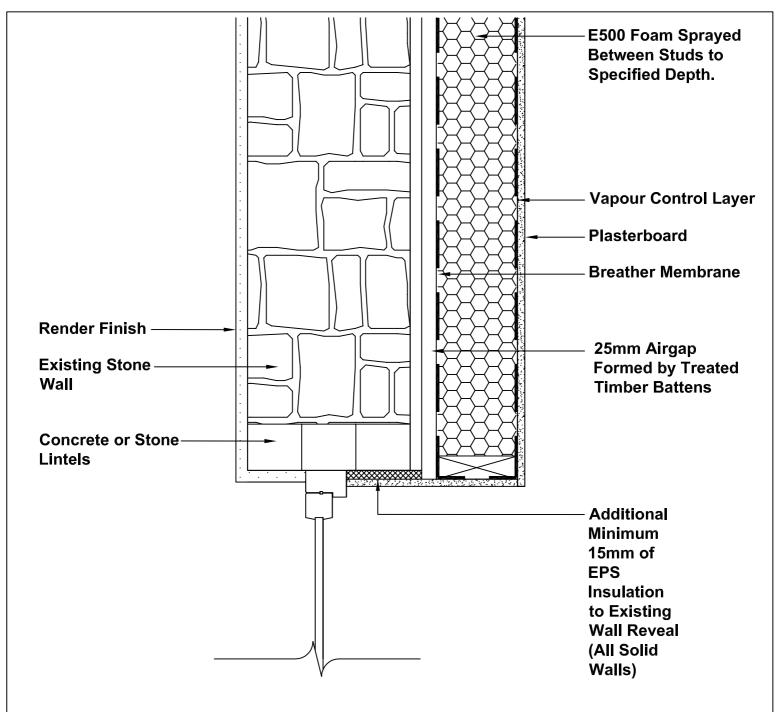
INTERNAL DRYLINING OF EXISTING MASONRY WALLS (VERTICAL SECTION AT LINTEL)
