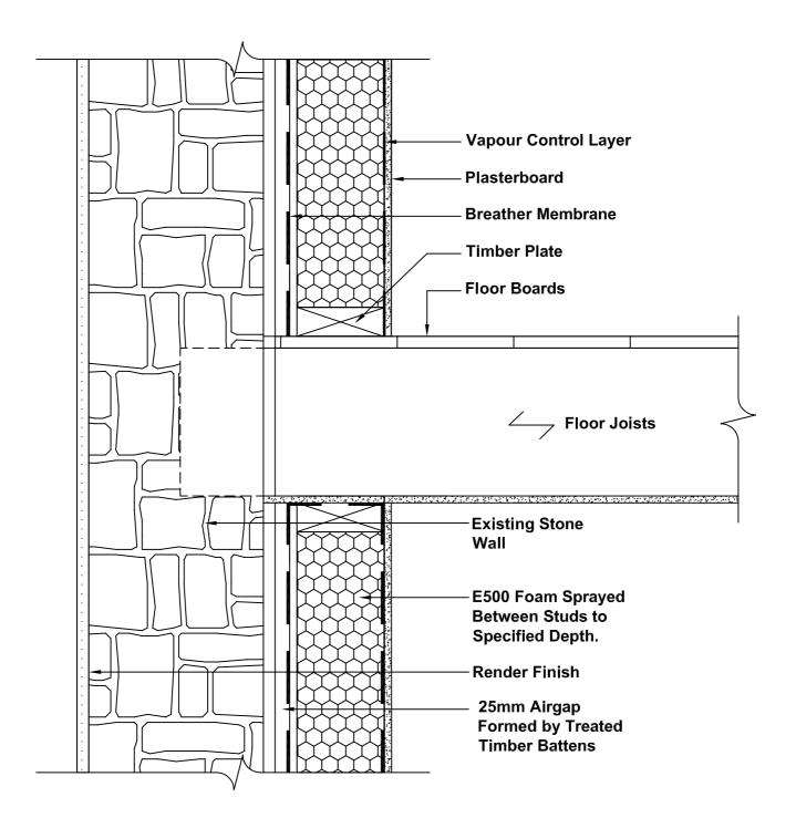
INTERNAL DRYLINING OF EXISTING MASONRY WALLS (VERTICAL SECTION - INTERMEDIATE FLOOR WITHIN A DWELLING)
