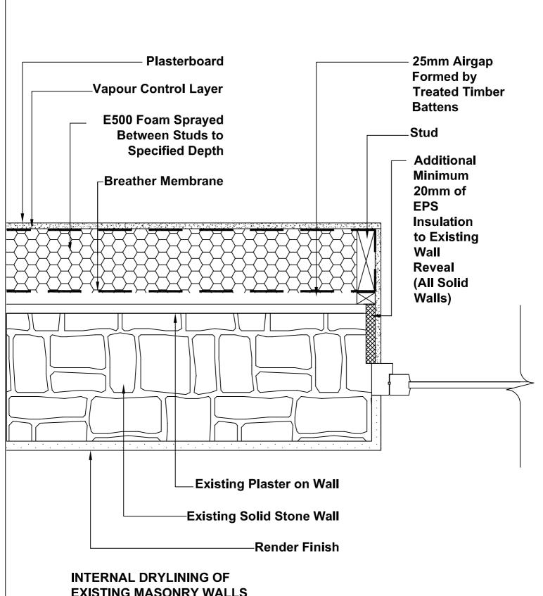
**EXISTING MASONRY WALLS** (PLAN SECTION AT JAMB)
